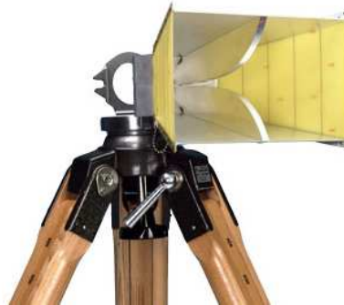
Figure 42 – Antenne cornet (modèle R&S HF906 1 – 18 GHz) [ http://www2.rohde-schwarz.com/en/ ]
