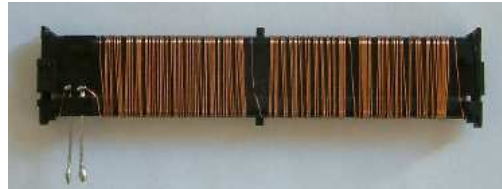
Figure 23 – Antenne ferrite (n = 160 tours, \mu_r = 60 , L = 820 \mu\text{H} ) [Brzeska]
