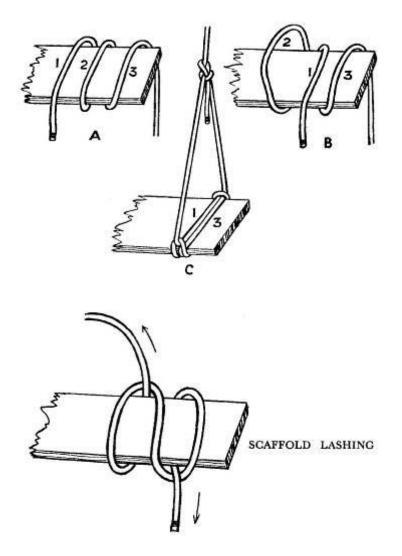
Probably the best method, however, is to make use of the scaffold hitch. Lay the short end of the rope over the plank leaving enough hanging down to tie to the long rope finally. Wrap the long end loosely twice round the plank. Carry rope 1 over rope 2 and place it between 2 and 3. Carry rope 2 over ropes 1 and 3 and over the end of the plank. Take up the slack by drawing on the two ends of the rope, and join the short end at a convenient distance above the plank to the longer with a bowline.
