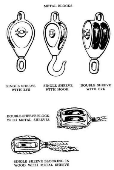
In general, it is wise to use the lightest blocks obtainable, so that you can use lighter ropes, and it is worth remembering that a very heavy block has to be supported, which materially affects the whole of the structure on which you are using it.
