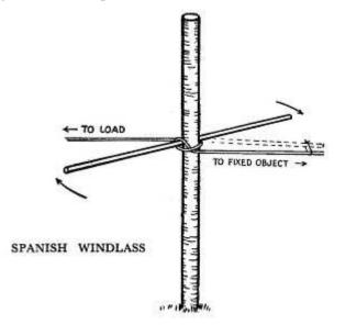
When a Spanish windlass is used for tightening up the hawser of a ropeway, it is only a temporary expedient and should not be used on ropes that are to take a great weight, as it weakens the rope considerably. In this case it is possible to drive the first spar into the ground, and to lash the second spar to the rope to keep it in position when sufficient strain has been obtained.
