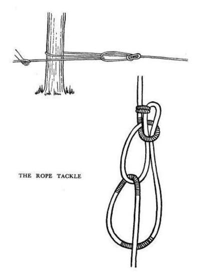
Let us assume that we are trying to tighten the runway of a light monkey bridge. We would bend one end of the rope in which we are going to make the tackle on to the end of the rope
