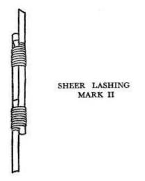
*Frapping.* – Having made the turns, firmly but not too tightly, frap twice by taking turns between the two spars and going round the lashing turns, finishing with a clove hitch on the
