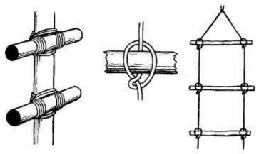
ROPE LADDER USING MARLINE SPIKE HITCHES
