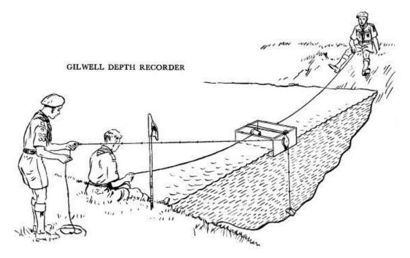
An improved model will have a continuous line from one bank to the other so that the apparatus can be manoeuvered accurately to any point on the measuring line.
