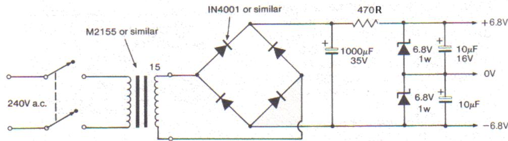
These two circuits show typical use of zeners in power supply circuits. The circuit below is designed to give increased current capacity. It will supply up to 1A with suitable heatsinking of the transistors.
