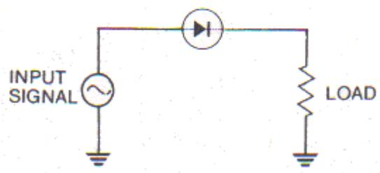
Simple diode rectifying circuit.
