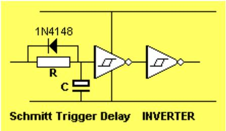
The following circuit produces a PULSE (a LOW pulse) when the input goes HIGH:
