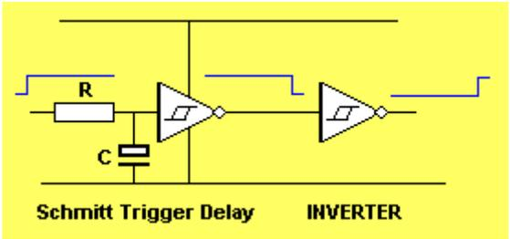
If a diode is added across the input resistor, the capacitor "C" will be discharged when the input goes low, so the "Delay Time" will be instantly available when the input goes HIGH:
