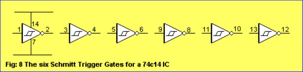
Fig: 8 The six Schmitt Trigger Gates for a 74c14 IC
