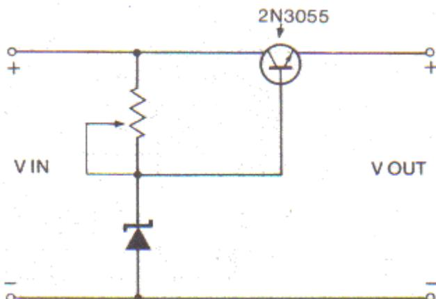
The output voltage of this circuit will be equal to the zener voltage minus the base-emitter voltage of the transistor (approx. 0.7V).
