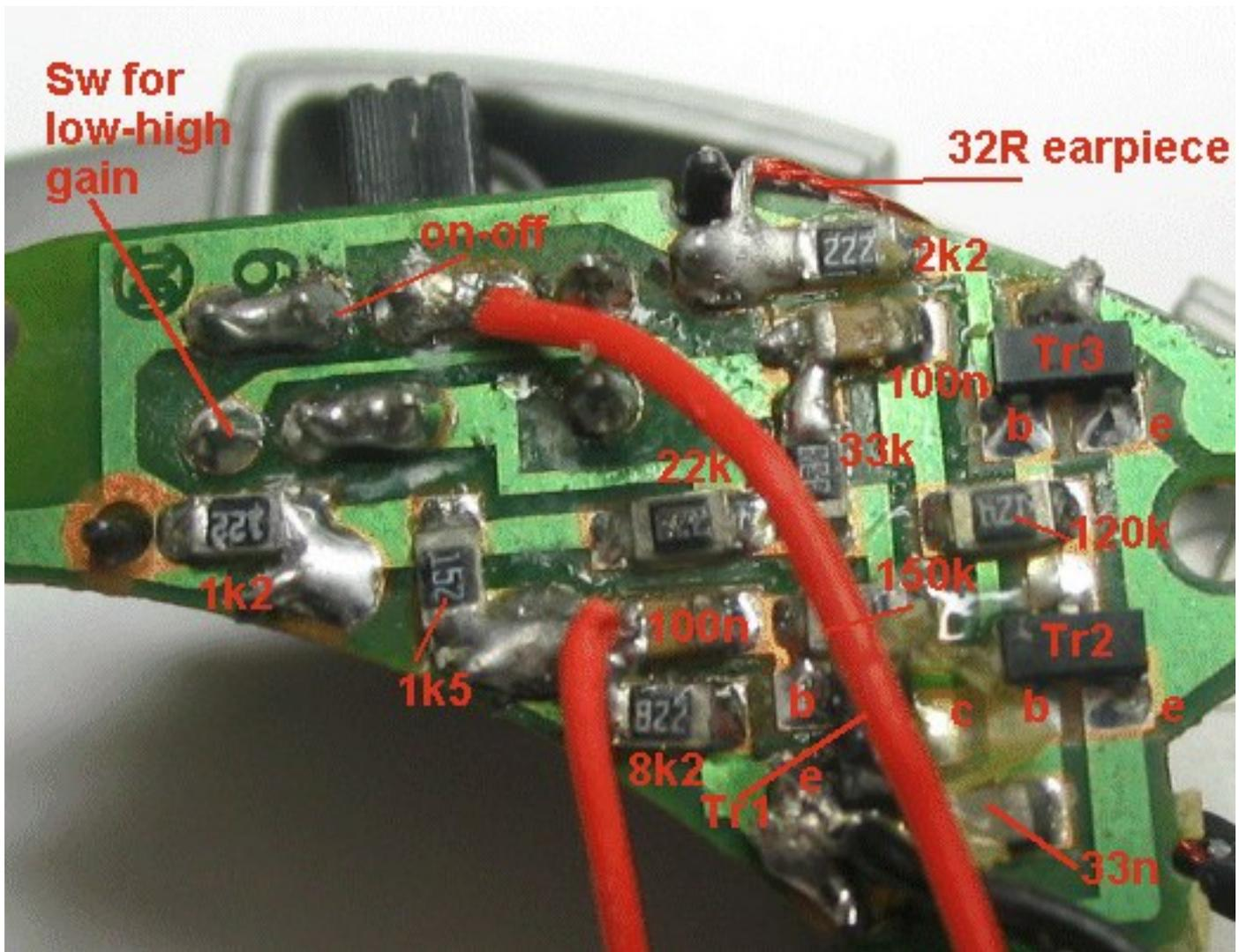
The surface-mount 3-Transistor amplifier
