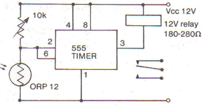
The 555 can supply current up to 200mA, so the relay type is not critical. Any with a coil resistance from 100-280 ohms would be suitable.
