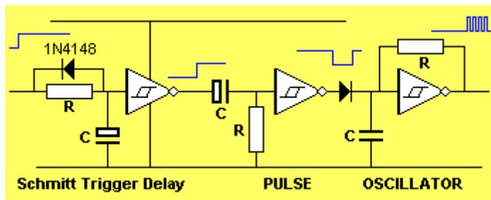
The oscillator above can be set to produce a 100Hz tone and this can activate a 2kHz oscillator to produce a 2-tone output. A "jamming diode" is needed between the third and fourth gates to allow the high-frequency oscillator to operate when the output of the low-frequency oscillator is HIGH.
