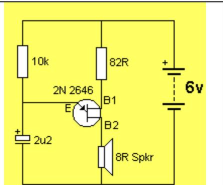
The output of the oscillator is a sawtooth. The higher the supply voltage, the lower the output frequency.
