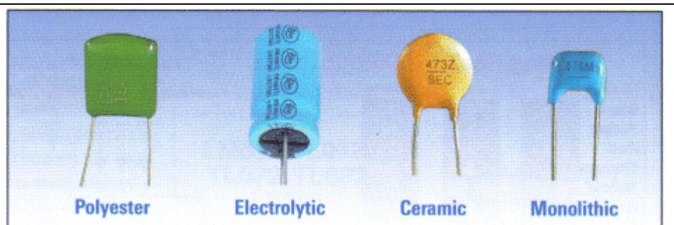
A capacitor works on the principle of having two conductive plates which are very close and are parallel to each other. When a charge is applied to one plate of the capacitor, the electrons will generate an approximately equal, but opposite charge on the other plate. Capacitors will pass AC current, but will block DC current. A capacitor can also be used to smooth voltage ripple, as in DC power supplies. Capacitance is measured in Farads (F).
