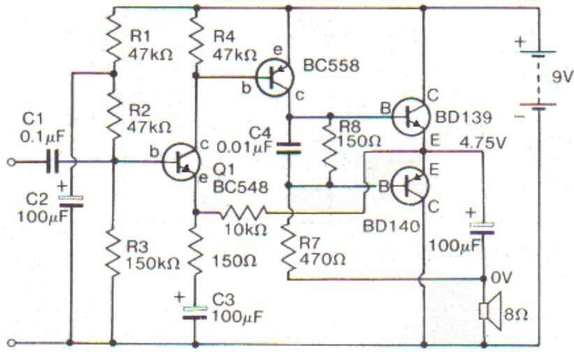
The circuit is for a low power amplifier using a BD139/140 pair in the output stage. The amplifier has a gain of 66. It needs 100mV input for full output, which is approximately 500mW into 8 ohms.
