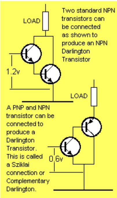
The Darlington Pair uses a pair of transistors coupled together as an emitter follower so that the emitter current of the first transistor flows through the base/emitter junction of the second transistor. The resulting current gain of the transistor pair is found by multiplying the current gain of the transistors together. The resulting current gain is very high and the input impedance of such a stage is very high.
