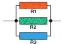
$$R_{\text{Total}} = \frac{1}{\left(\frac{1}{R_1} + \frac{1}{R_2} + \frac{1}{R_3} + \text{etc .....}\right)}$$
