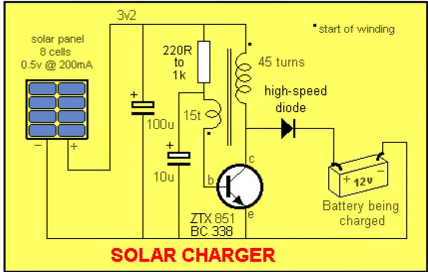
This solar charger can be used to charge a 12v battery from any number of solar cells. The circuit automatically adjusts for any input voltage and any output voltage. See Talking Electronics website for the full project.
