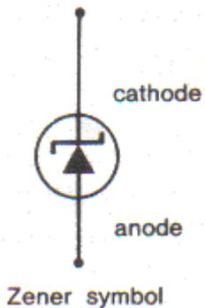
Unlike conventional diodes, zener diodes are deliberately intended to be used with the anode connected to a negative potential (or 0v) and the cathode connected to the positive potential. When connected in this manner, zener diodes have a very high resistance below a certain critical voltage (called the zener voltage). If this voltage is exceeded, the resistance of the zener drops to a very low level.
