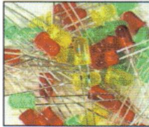
The LED's legs are called anode and cathode. The anode is the leg that needs to be connected to the positive of the power source. Normally a LED has different lead lengths to identify which is the positive lead. However if the leads have been trimmed, the cathode is denoted by a flat face on round LEDs or the larger internal part of the LED.
