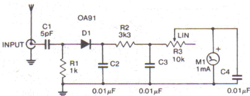
The circuit is an RF monitor meter suitable for measuring the strength of a signal from transmitters. You could use it to measure the effectiveness of different antennas for example. It works in much the same way as the crystal set, but without the tuned circuit. The meter M, will indicate the strength of the 'carrier'. Modulation of the carrier i.e. signal on the carrier, will cause the reading to vary. M, is not critical, and any meter of 1mA or better sensitivity will be suitable.
