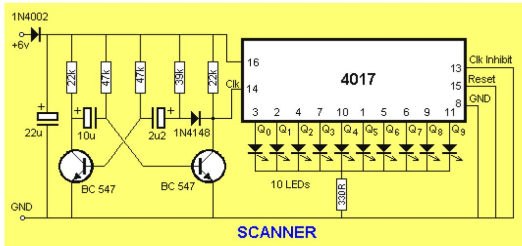
The 10 LEDs on the SCANNER turn on one-at-a-time, from left to right
