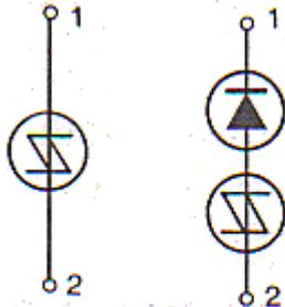
SYMBOL OF ASYMMETRICAL AC TRIGGER SWITCH (ST4) AND EQUIVALENT CIRCUIT
