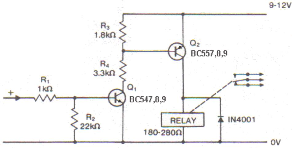
The circuit will work with any relay with a coil resistance higher than 180 ohms and a pull in voltage of less than 12v.
