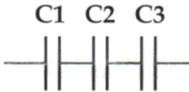
$$C_{\text{Total}} = \frac{1}{\left(\frac{1}{C_1} + \frac{1}{C_2} + \frac{1}{C_3} + \text{etc} \dots\right)}$$
