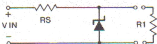
If the Zener diode is rated at 5.6V and the applied voltage is 8.0V, then with no load applied, the output voltage across R1 will be 5.6V and the remaining 2.4V will be dropped across R<sub>s</sub>. If the input voltage is changed to 9.0V, then the voltage across the Zener will remain at 5.6V. In practice, the voltage across the Zener will rise slightly due to the 'dynamic resistance' of the zener.
