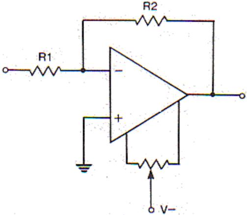
Output offset null circuit for op amps with internal nulling provisions.
