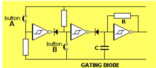
The second diode is called the **gating diode**. When the output of the second inverter is LOW, the capacitor is prevented from charging as the diode will not allow it to charge higher than 0.7v, and thus the oscillator does not operate. When the output of the second inverter is HIGH, the capacitor is allowed to charge and discharge and thus oscillator will produce an output. If the push buttons can be placed together, the circuit can be simplified to:
