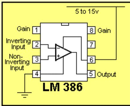
The LM 386 is an 8-pin Audio Power Amplifier
