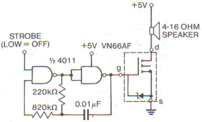
The addition of a VFET driver transistor following a CMOS oscillator makes a very efficient and simple audio alarm. As well as this it will drive a low impedance speaker directly.
