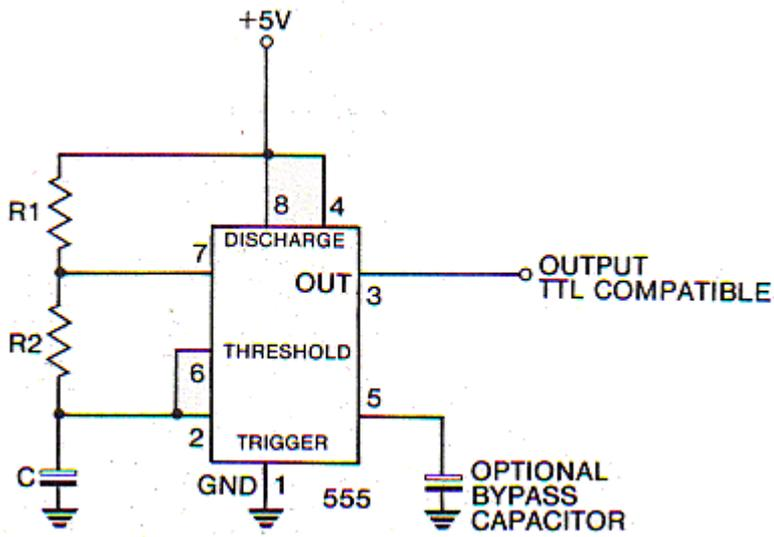
If  $R_2$  is made large compared to  $R_1$ , output is low but symmetry of waveform is high.
