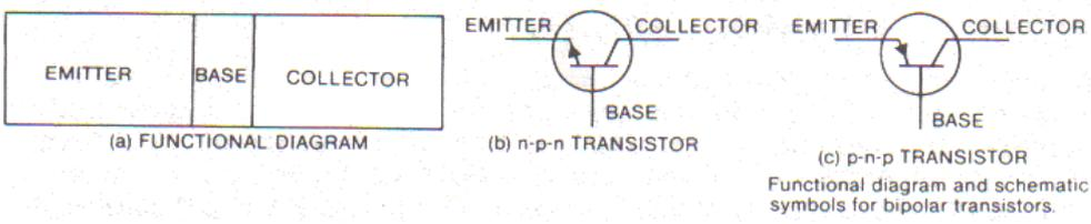
Functional diagram and schematic symbols for bipolar transistors.
