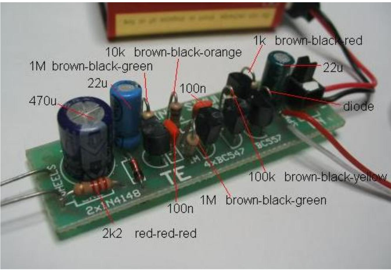
A realistic steam sound can be generated with a 4-transistor directly-coupled amplifier connected to a small speaker. The “white noise” is generated by the breakdown across the junction of a transistor and it is activated by a switch made up of contacts touching the wheel of one of the carriages. As the train speeds up and slows down, the sound corresponds to the movement. See Talking Electronics website for the full project.
