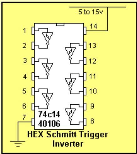
This chip is known by a number of identities. 74C14. It is also marketed as 40106, 40014, and 74HC14. These are all CMOS chips and are characterised by low current consumption, high input impedance and a supply voltage from 5v to 15v. (Do not substitute 7414 or 74LS14. They are TTL chips and operate on 4.5v to 5.5v and have low impedance inputs.)
