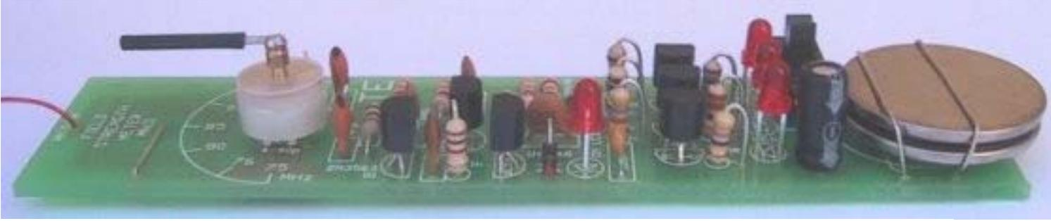
A field strength meter is a very handy piece of test equipment to determine the output of a transmitter. Talking Electronics website describes a number of Test Equipment projects to help with developing your projects.
