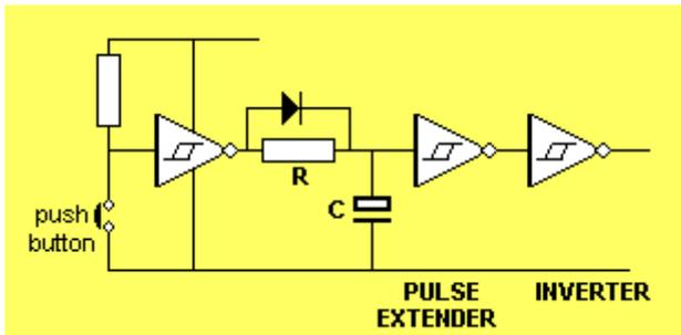
To produce a pulse of constant length, (no matter how long the button is pressed), the following circuit is needed:
