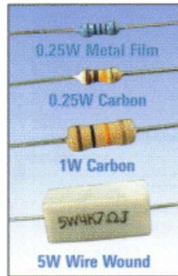
A resistor will limit the current flow through itself to a calculable value based upon its resistance and the applied voltage (see Ohms Law). This means a resistor can be used to run a low voltage device from a higher voltage power supply by limiting the required power to a predetermined level. Resistors are not polarity sensitive.
