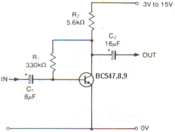
This circuit will operate on any supply from 3v to 15v. Using a 9v supply, the circuit gives a voltage gain of 46dB (200 times), frequency response within 3dB from 30Hz to 100kHz, input impedance of 1.5k ohms and an output impedance of 5.6k ohms. The base bias resistor R<sub>1</sub> gives sufficient negative feedback to compensate for the large variation of h<sub>FE</sub> values in individual transistors and for variations in supply voltage.
