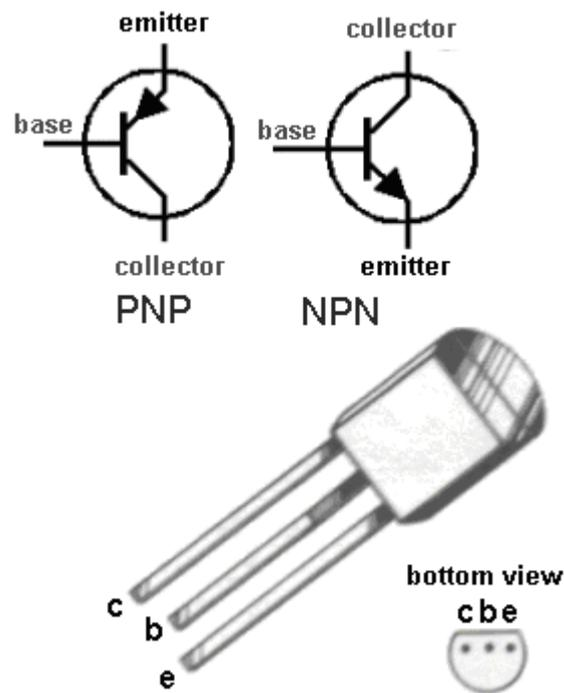
Low frequency, general purpose small signal transistors widely used in audio, switching and television circuits. The BC547-9 series and BC557-9 series are functionally identical to the common BC107-9 series. All have a maximum power dissipation of 500mW. They have essentially similar specifications and can generally be substituted for one another (within the PNP and NPN groups of three each). All devices are housed in standard TO-92 plastic packages.
