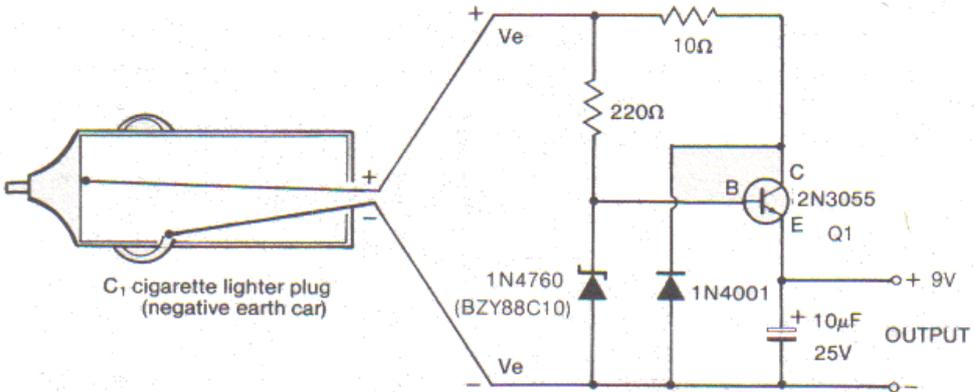
The output will drive transistor radios, cassette players etc. If the current drain is over 500mA, it is a good idea to put a heat sink on Q<sub>1</sub>. Mounting the converter in a metal box with Q<sub>1</sub> on the lid (but insulated from it with a mica washer) will act as a good heatsink.
