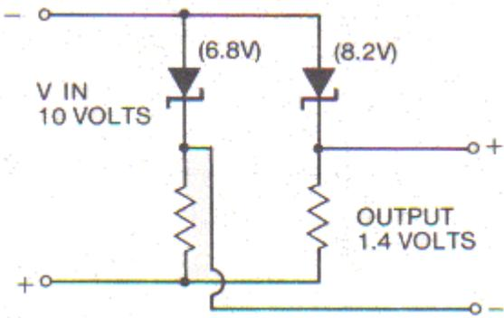
It may also be necessary at times to provide a regulated voltage lower than that normally available from a zener diode. These voltages may be obtained by using the difference between two pairs of zeners. This is shown in the circuit below. As a bonus, the temperature compensation of this circuit is excellent, since both zeners tend to drift in the same direction, maintaining the voltage difference.
