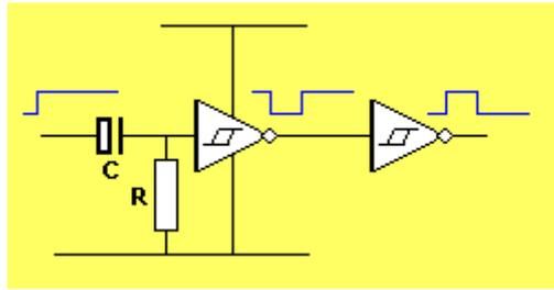
To produce a pulse after a delay, the following circuit can be used:
