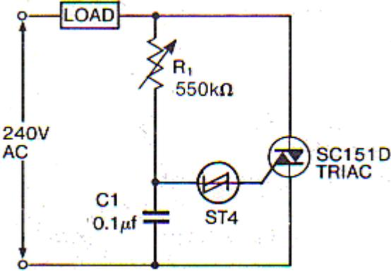
This easy-to-build controller is ideal for dimming lights, and controlling the output of electric heating type appliances. The light or heater element etc is placed where the 'LOAD' is marked on the circuit.
