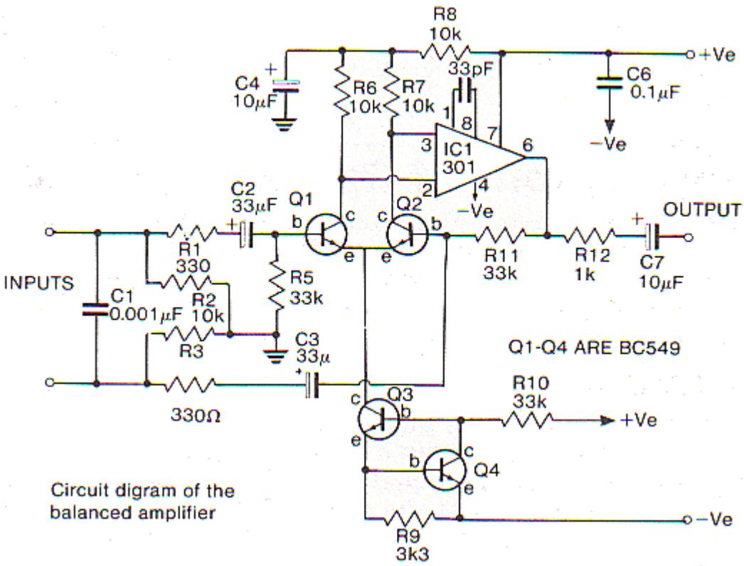
Circuit diagram of the balanced amplifier
