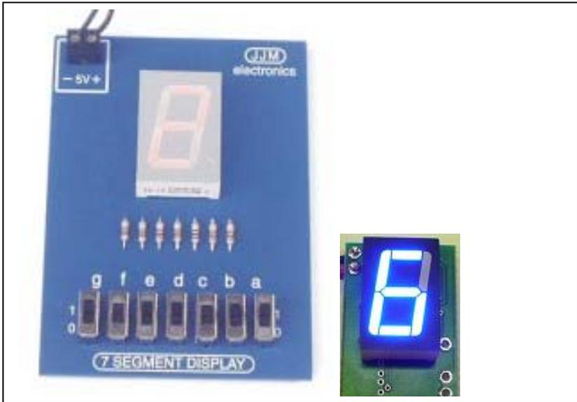
The project above from JIM turns on each segment of the display to show how each letter and number is produced. The second photo is a white 7-segment display.
