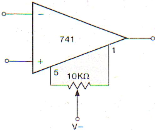
This can be important in DC circuits or where a high impedance feedback resistor is used. A 10k ohm variable resistor is connected between pins 1 and 5 (of the 8 pin package) and the wiper is taken to - supply.
