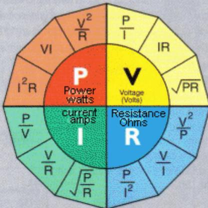
Using this formula wheel it is possible to calculate power, volts, amps or resistance for a given problem. i.e. if you have two of the variables, for example power and volts, it is possible to find the amps in a circuit.
