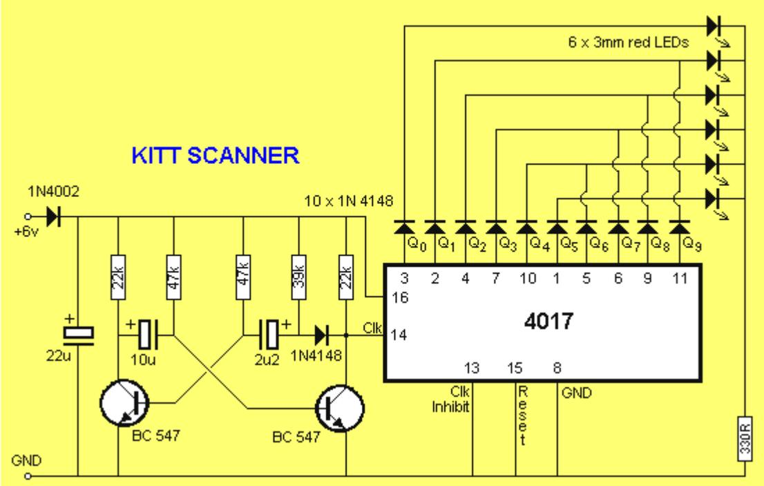
6 LEDs on the KITT SCANNER scan back and forth similar to the lights on the front of the KITT car in the movie.
