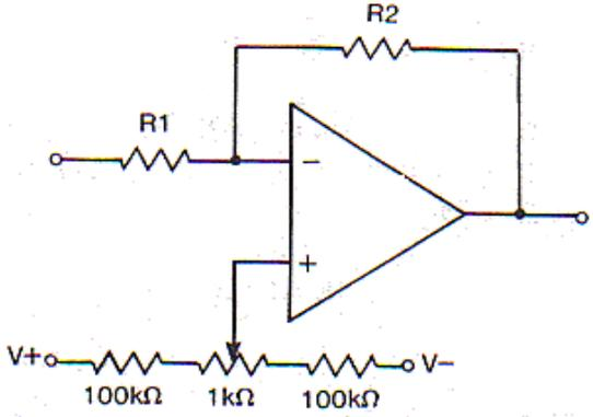
Output offset null control for op amps.
