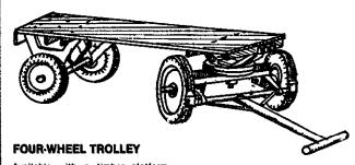
Available with a timber platform (180 x 80cm or 200 x 100cm), this wagon is able to carry loads of up to 750 kg. It is equipped with a wide T-shaped handle with a cross-barfitted to the front wheels which are attached to the main chassis by a bodge arrangement. The wheels are littled with pneumatic tyres.
