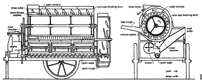
Schematic drawing of an axial flow thresher.
