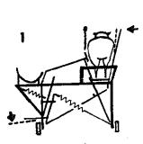
Sheep enters race and is secured in a cage. All movements of the machine initiated by foot levers.
