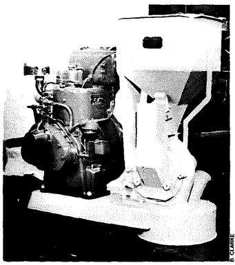
Small grain hammer mill with diesel drive.
