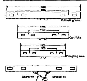
Trens can be lengthened or shortened to accommodate differences in strength of oxen.
