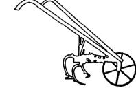
for different types of work if necessary. The cultivator is available with various attachments for weeding, hilling, ridging or furrowing, it has a capacity of 4-5 hah and a working width of 250-350mm. The net weight of the cultivator is 17kg.
