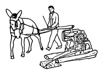
ANIMAL POWERED MONOLIFT PUMP ANIMAL POWERED MONOLIFT PUMP This rotary pump is an adaptation of the Monolift borehole pump. Suitable for maximum lifts from 30 to 110m depending on type and number of animals used. Maximum output ranges from 1.2 to 4.5m<sup>2</sup>/h.
