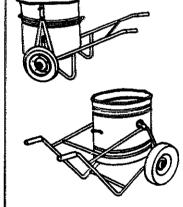
The galvanized container pivots on a horizontal axis and is manufactured with a pouring lip. Container capacities available are 100 litres and 150 litres. The chassic is of tubular steel and has two wheels with solid rubber, or, (for models produced by G. Elt), pneumatic tyres.
