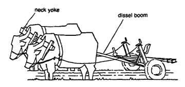
Pair of animals with neck yoke and dissel boom attached between them and to multi-purpose wheeled tool carrier.
