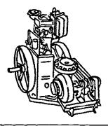
VIJAY PUMPSETS These consist of a vertical water cooled single-cylinder diesel engine from 5 to 10hp coupled either directly or by belt drive to a variety of centrifugal pumps — self priming, enduction, split casing and volute types, shown right. Total head range from 6 to 26m with outputs from 135 to 36m<sup>3</sup>/h respectively. Electric motor driven options also available.
