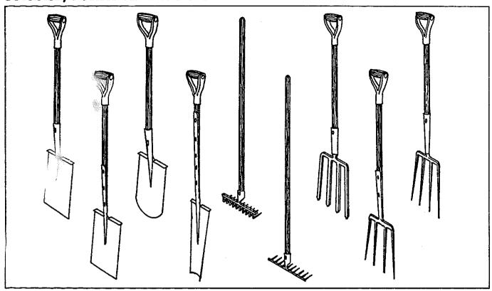
From left: solid socket treaded spade; strapped treaded spade; open socket treaded round nose spade; strapped treaded drainage spade; shaped-tine rake; garden rake; tang and ferrule broad-tine digging fork; strapped fork; solid socket digging fork.
