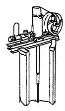
'SIRIUS' DEEP WELL PUMP The electric motor-driven deep well lift and force pump, illustrated right, is suitable for lifts of up to 50m or more and for forcing up to 80m. Five cylinder sizes available, from 60 to 120mm with outputs from 0.6 to 4m³/h.
