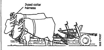
Pair of animals with three-pad collars hitched to multipurpose tool carrier with horizontally held boom, spacers and swingle tree.
