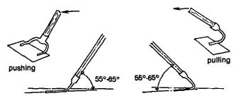
Fig.1 Pushing and pulling hoes, showing working angles.
