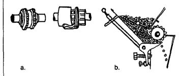
Fig.7 a. Fluted roller and slide roller-feed mechanisms, b. Seed roller.
