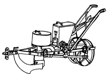
Fig.5 Single-row seed and fertilizer drill with Pitman drive.
