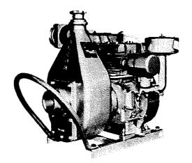
PORTABLE PUMP UNIT This steel bodied self-priming centrifugal pump, fitted with a pair of carrying handles, is available in two sizes, 51 and 76 mm outlet diameter. Connected by belt-drive to a 5hp diesel or optional light-weight petrol engine, they have maximum outputs of approximately 30 and 70m<sup>3</sup>/h at an operating head of 9m. Weight 120ko.
