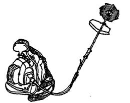
CLEARING SAW WITH KNAPSACK MOUNTED MOTOR
