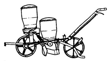
Fig.6 Chain and sprocket driven planter/fertilizer.
