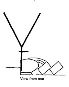
Fig.1 Three views of a mouldboard plough at its correct setting.
