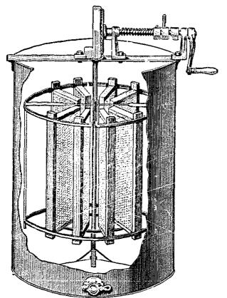
Radial extractor for spinning honey out of the cells in the comb.
