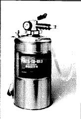
The stainless steel tank holds about 4kg of powder. A compressed air source is used to pressurise to about 7kg/cm². On squeezing lever up to 2kg of powder is released in 20 seconds. The blower weighs only about 3kg it is supplied with a 7.5m flexible hose, it is particularly useful for injecting insecticides into crevices and roof spaces of warehouses.
