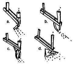
Fig.3 Seed Coulters: a. cultivator type share, b. drag share, c. double disc share, d. goose-foot share (for strips).
