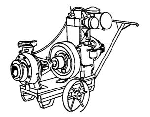
100mm (pump outlet diameter). Total head ranges from 9 to 18m with corresponding cutputs from 144 to 40m³/h. Weight 166kg. Larger twincylinder model, DE.14 has approximately double the capacity.
