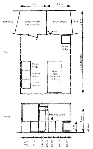
A small general-purpose building with a single stand can comfortably handle 400-600 sheep. Blade shearing, portable machines or fixed equipment can all be considered.
