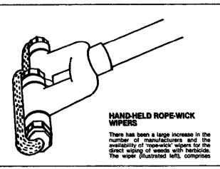
two nyion braided ropes fed by a horbicide reservoir in the tubular handle. Note: the nuts can be tightened or slackened to control flow.
