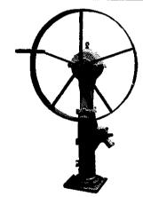
mainly cast iron, double flywheel model is achieved by twin connecting rods and crosshead. Fitted with balance weights, the handwheels are extra wide for optional belt drive. Extractable or non-extractable cylinders available in eight sizes from 57 to 102mm for matching maximum heads from 53 to 12m. Corresponding outputs 13 and 41 litres/min at 40 strokes, the former with two operators.
