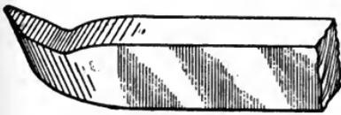
Fig. 125. Tool for Finishing Wrought Iron and Steel
