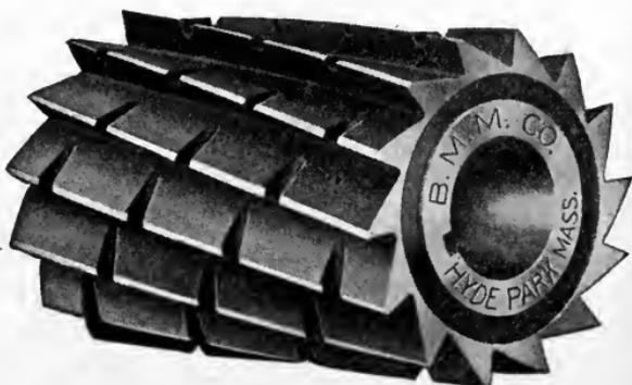
Fig. 206. Spiral Cutter with Nicked Teeth for Heavy Cuts
