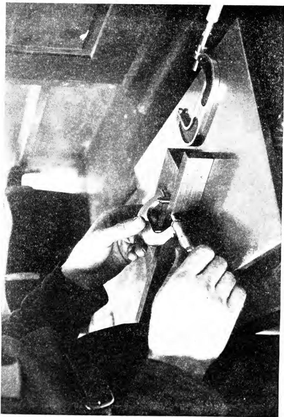
MAKING ACCURATE MEASUREMENTS WITH MICROMETER CALIPER
