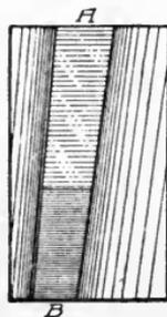
Fig. 159. Square Thread Tool Showing Inclination of Thread to Body
