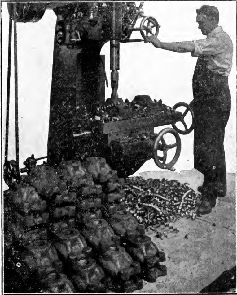
Fig. 348. Baker Driller Driving 2½-Inch Drill through Drop-Forged Wrought-Iron Saddles
