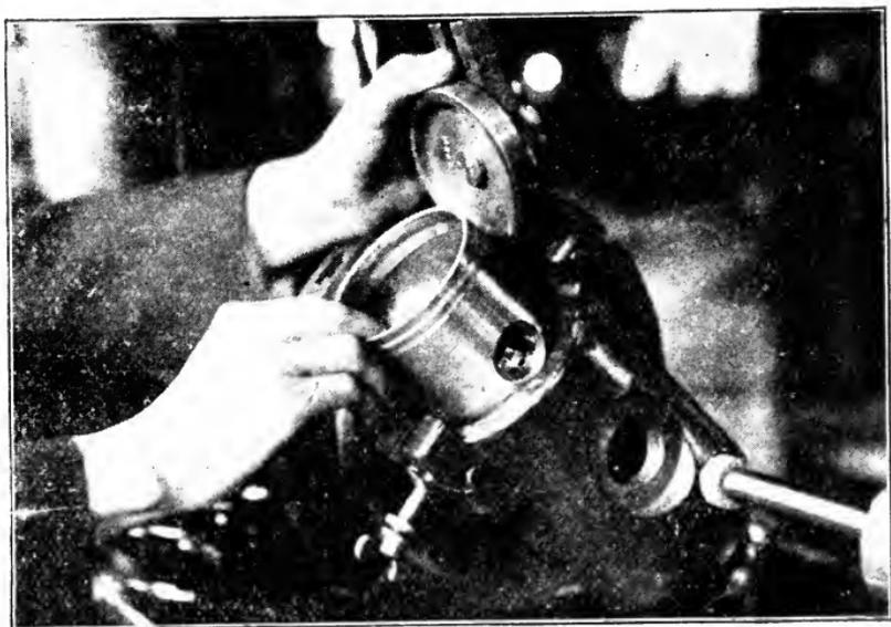
Fig. 337. Charging Grinding Jig Shown in Fig. 336
