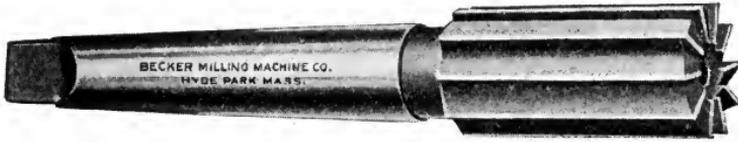
Fig. 215. Ordinary Form of End Mill
