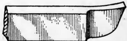
Fig. 127. Cutting-Off or Parting Tool
