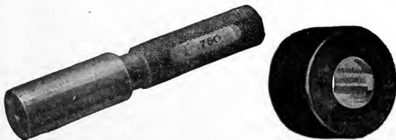
Fig. 35. Typical Plug and Ring Gages
