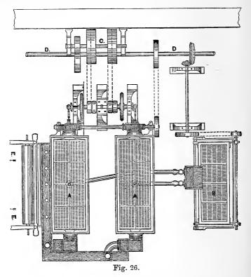
the apparatus is supplied with driving gear, bellows, regulating boxes and spouts, as necessary. The firm also supply these strainers with White's patent discs, and Annandale and Watson's arrangement. A A are two revolving strainers, as applied to the paper-machine, showing gear-
