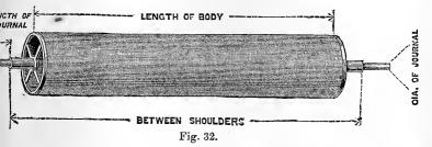
the moist pulp correspond with those of the machine-wire on the under surface. By this means paper known as "wove" paper is produced. A dandy-roll of this character is shown in Fig. 32. "Laid" paper, as it is
