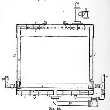
off, the spent liquor is run off, and hot water then run into the boiler, steam again turned on, and the boiling kept up for about twenty minutes to half an hour, at the end of which time the steam is shut off and the blow-pipe opened. As soon as the steam has blown off, the washing water is run off by the bottom pipe, and the grass allowed
