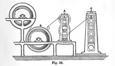
sists of a damping apparatus A (Fig. 38) which is placed between the last drying cylinders B of the machine and the glazing calenders c. The damping-rolls consist of
