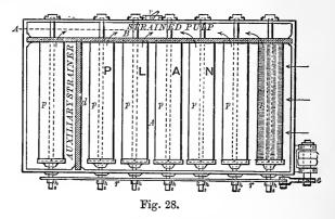
cleaned. One or more fans are fitted in these boxes, and are put in motion from the outside, so as to cause what is called "suction" through the strainers. One or a number of such boxes are fixed into a vat, the open ends discharging the pulp which has passed through the strainers
