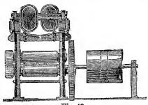
which is shown in Figs. 49 and 50, is also made by the firm referred to, and consists of two hammered iron rolls, each about twelve inches in diameter, of any suitable length, carefully turned and carried by strong cast-
