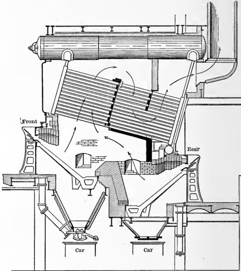
Fig. 367. — Double-furnace Boiler.
