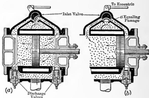
Fig. 437. — Dry Air Pump with Equalizing Passage.
