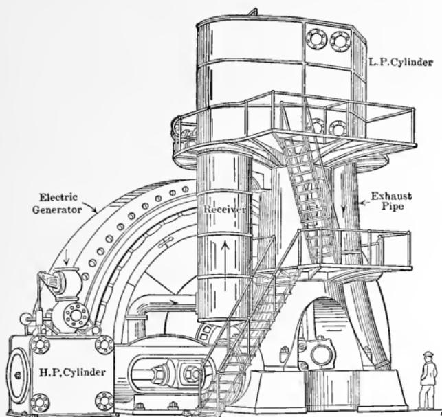
Fig. 110. — Angle-Compound Engine.
