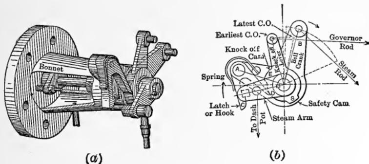
Fig. 187. — Steam Gear—Corliss Engine.
