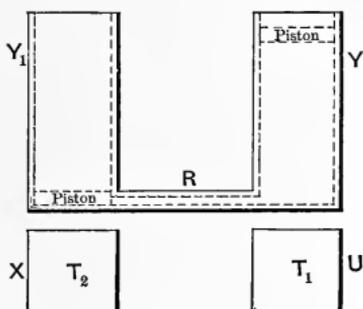
Fig. 23. — Machinery of Constant-Volume Regenerative Cycle.
