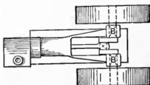
Fig. 106. — Center-Crank Engine.
