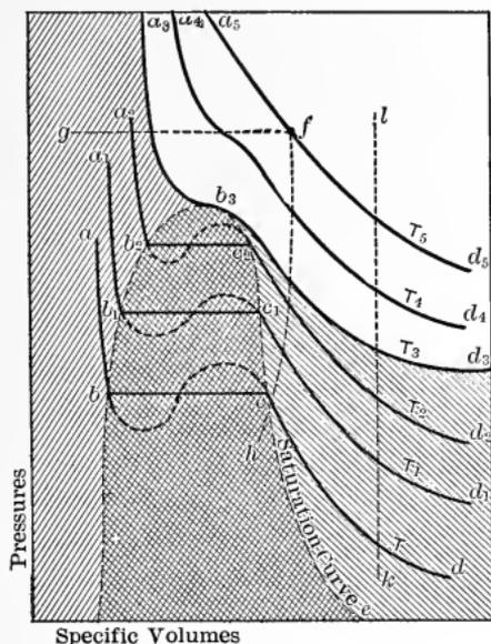
Fig. 34.—Isothermals of Material in Liquid, Vaporous and Gaseous States.
