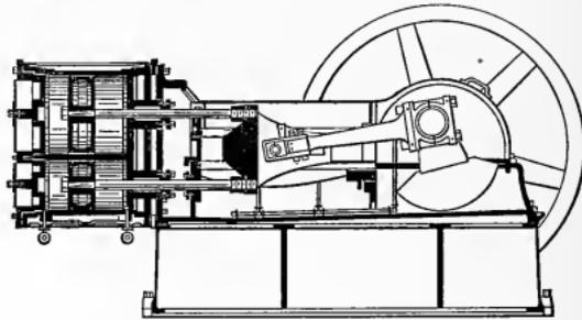
Fig. 109. — Duplex-Compound Engine.
