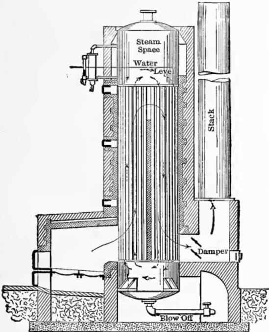
Fig. 364. — Wickes Type of Boiler.
