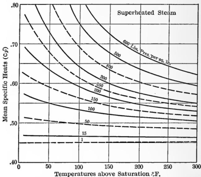
Fig. 40. — Variation of Mean Specific Heat  $\bar{C}_p$  of Superheated Steam.
