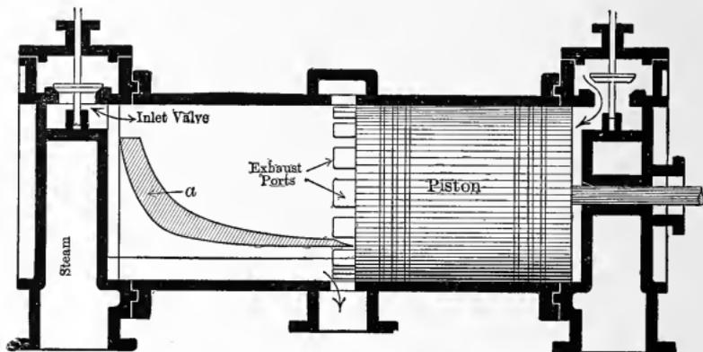
Fig. 96. — Unidirectional-Flow Engine.
