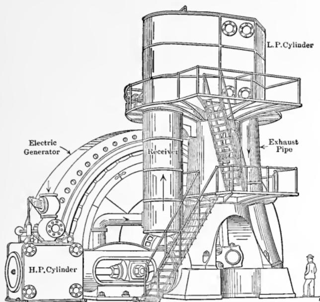
Fig. 110. — Angle-Compound Engine.
