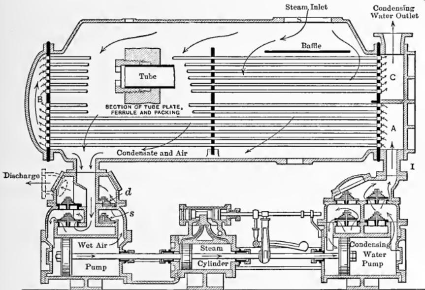
Fig. 433. — Double Flow Surface Condenser.
