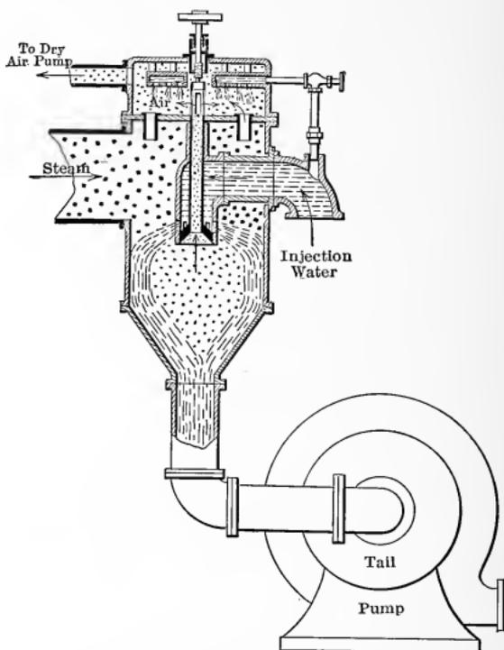
Fig. 431. — Condenser with Dry Air Pump.
