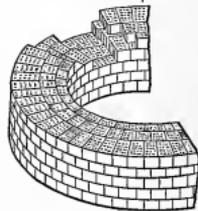
changes. By using special *radial brick* (Fig. 378), composed of suitable material, and commonly made perforated, (1) the lining may be omitted, (2) the shell may be thinner and of lighter weight, and (3) the foundation may be smaller; besides which (4) the construction is better and (5) can be more rapidly done than with ordinary brick. The tallest chimney in the world is of this type. It is located at Great Falls, Mont., and is 506 feet high with 50 feet diameter at the top.
