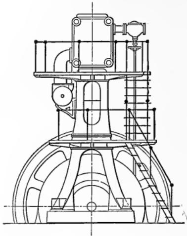
Fig. 101. — Vertical Corliss Engine.
