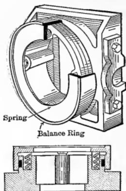
Fig. 156. — Valve with Balance Ring.
