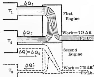
Fig. 19. — Energy Flow in Carnot Engine.
