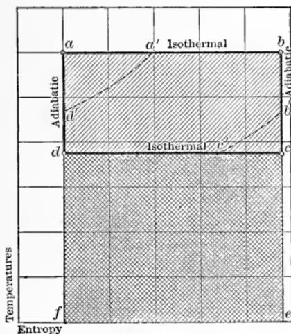
Fig. 21. —  $T\phi$ -Diagram of Carnot Cycle.
