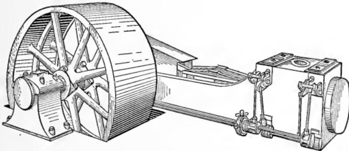
Fig. 100. — Medium-Speed Engine — Shaft Governor — Positive Cut-off.
