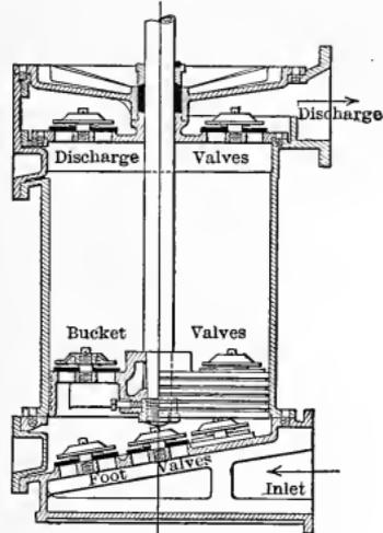
Fig. 438. — Wet Air Pump.
