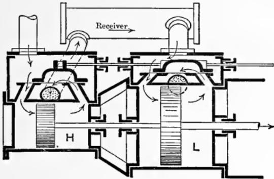
Fig. 107. — Tandem-Compound Cylinders.
