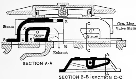
Fig. 151. — Double-ported Marine Valves.
