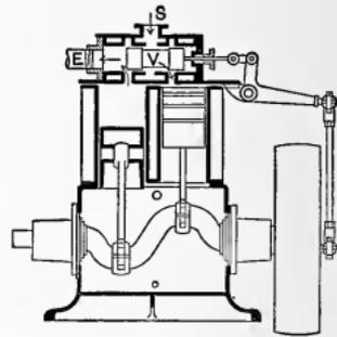
Fig. 102. — Vertical Twin-Cylinder, Single-Acting Engine.
