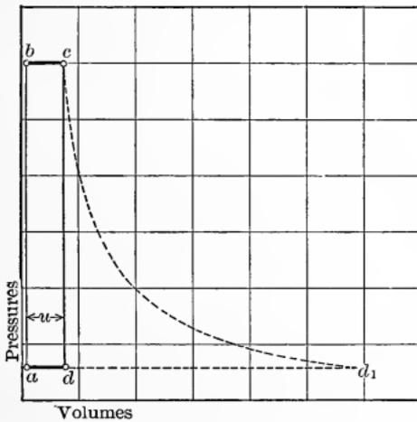
Fig. 62. — Cycle with Rectangular PV-Diagram.
