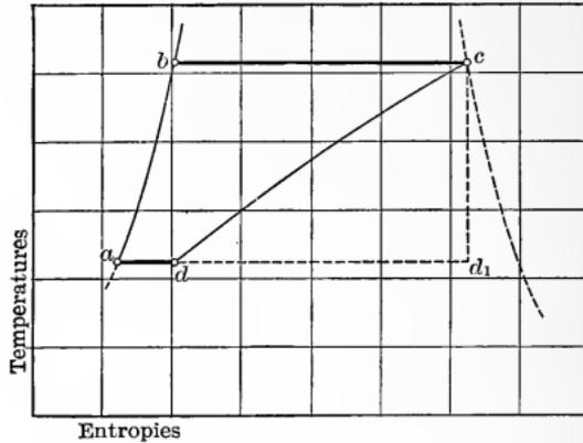
Fig. 63. —  $T\phi$ -Diagram for Rectangular PV Cycle.
