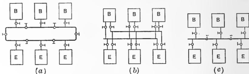
Fig. 450. — Steam Piping Arrangements.
