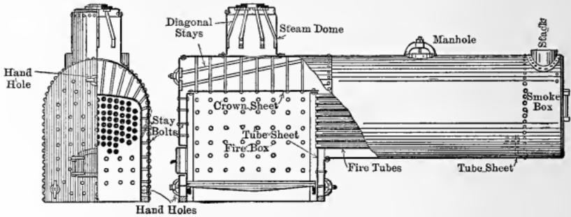
Fig. 354. — Locomotive Type of Boiler.
