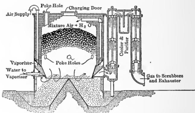
Fig. 393. — Down Draft Producer, Continuously Operated. (Akerlund Type.)
