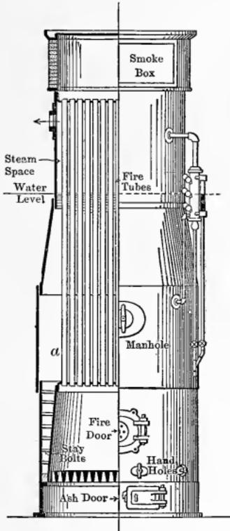
Fig. 353. — Tubular Boiler.
