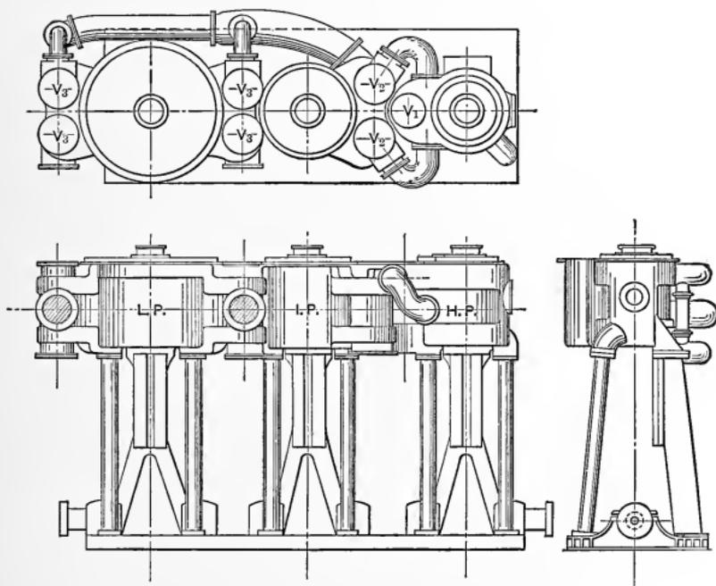
Fig. 111. — Vertical Triple-Expansion Marine Engine — Arrangement.
