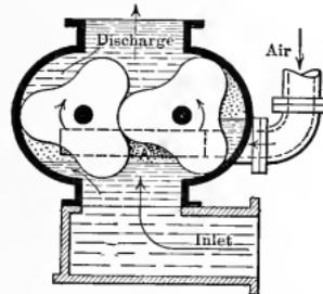
Fig. 440. — Rotary Type of Air Pump.
