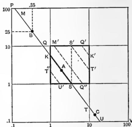
Fig. 14.—Checkerboard of Logarithmic Charts.
