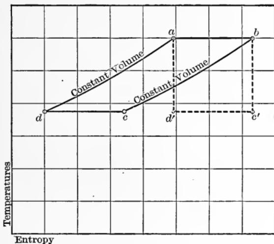
Fig. 24. —  $T\phi$ -Diagram of Constant-Volume Regenerative Cycle.
