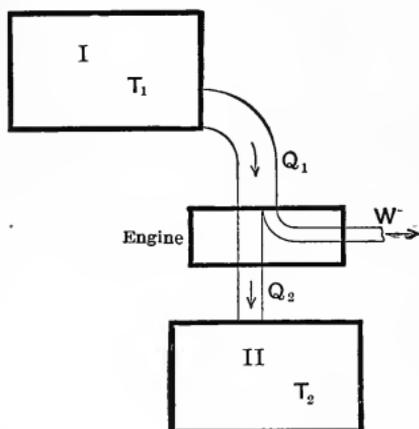
Fig. 1 — Diagrammatic Representation of a Heat Engine.
