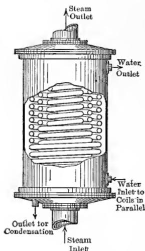
Fig. 423. Coil Heater.
