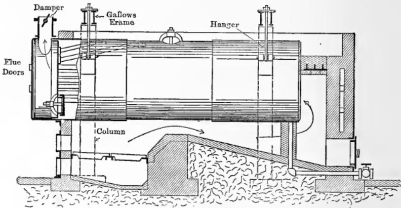
Fig. 358. — Horizontal Return Tubular Boiler with "Half Front."
