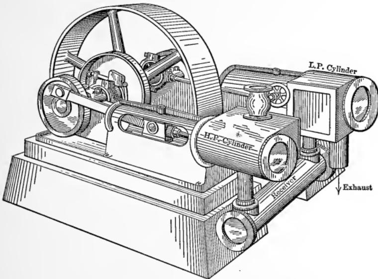
Fig. 108. — Cross-Compound Engine.
