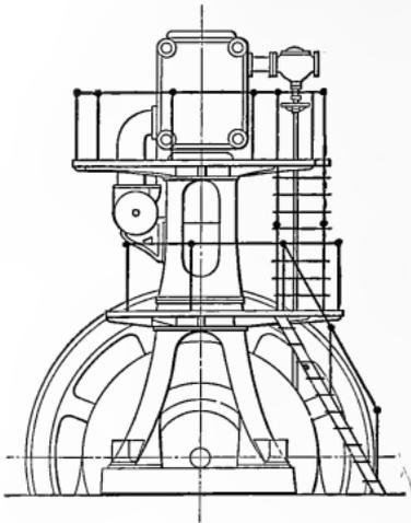
Fig. 101. — Vertical Corliss Engine.
