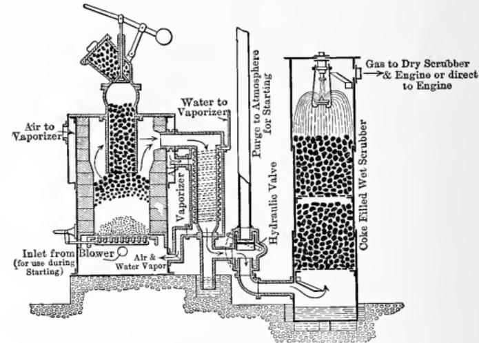
Fig. 391. — Up Draft Suction Producer.
