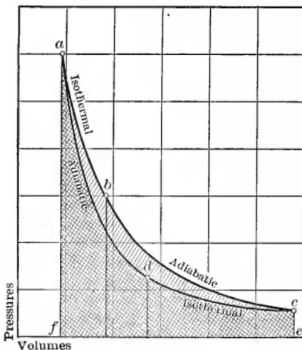
Fig. 18. — PV-Diagram of Carnot Cycle.
