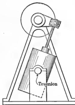
Fig. 104. — Oscillating Engine.
