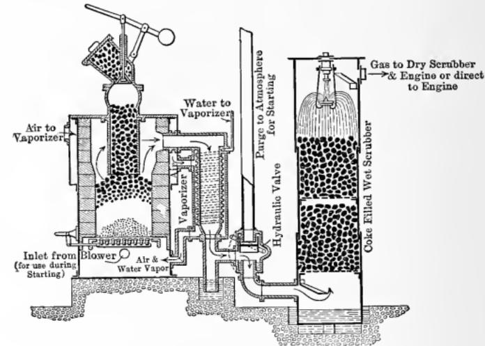
Fig. 391. — Up Draft Suction Producer.
