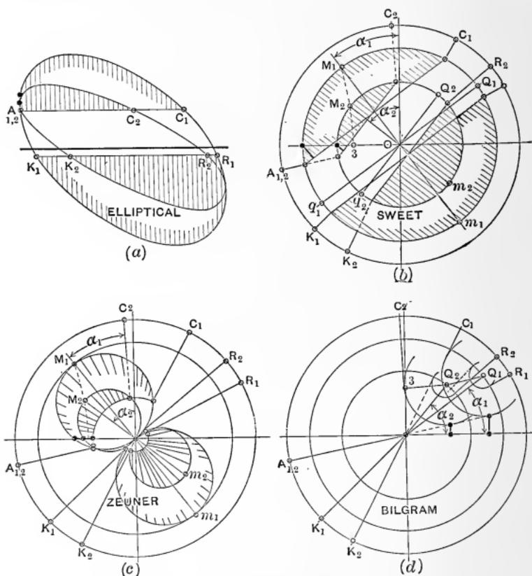
Fig. 162. — Valve Diagrams for Variable Eccentric Valve Gear.
