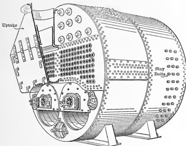
Fig. 356. — Scotch Marine Type of Boiler.
