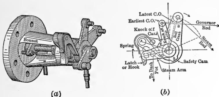
Fig. 187. — Steam Gear—Corliss Engine.
