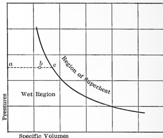
Fig. 32. — Saturation Curve for Water Vapor.
