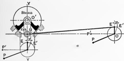
Fig. 181.—Oscillating Valve.
