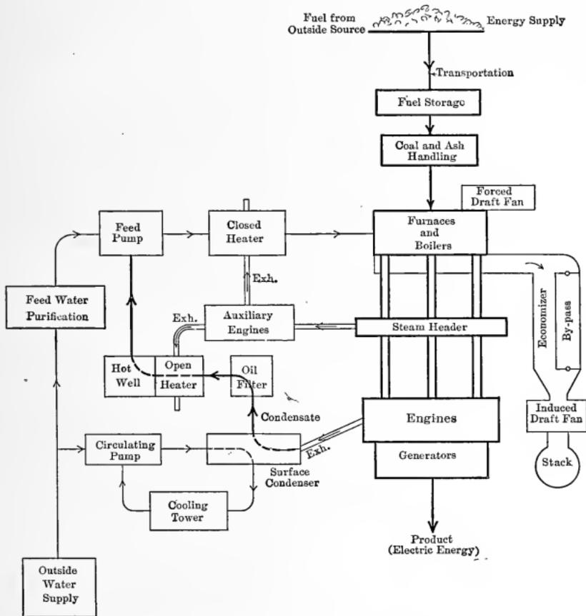
Fig. 444. — Elements of a Steam Power Plant.
