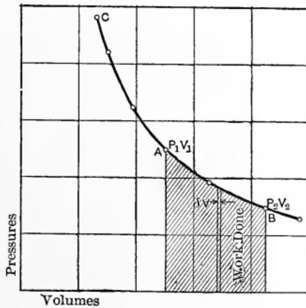
Fig. 9. — Isothermal Changes for Ideal Gases
