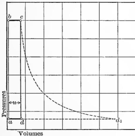
Fig. 62. — Cycle with Rectangular PV-Diagram.
