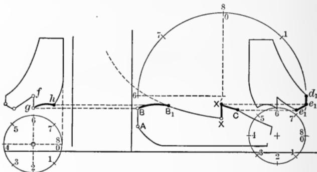
Fig. 224. — Low-pressure Cut-off later than Half-stroke.
