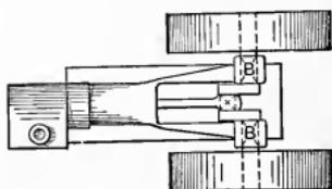
Fig. 106. — Center-Crank Engine.
