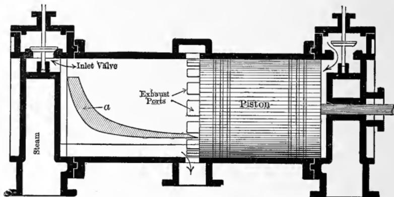
Fig. 96. — Unidirectional-Flow Engine.
