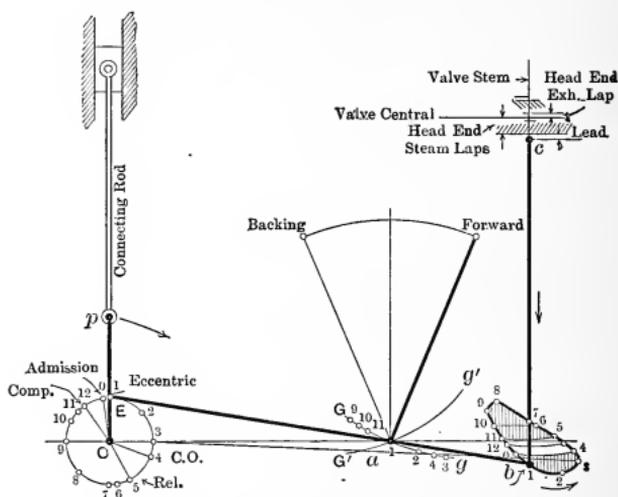
Fig. 199. — Marshall Type of Radial Gear.
