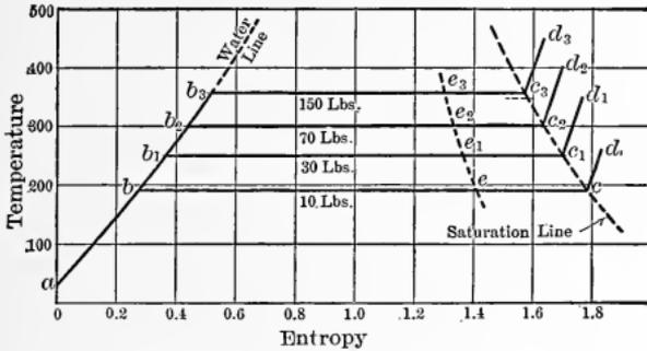
Fig. 33. — Tφ-Diagram for Water and Water Vapor.
