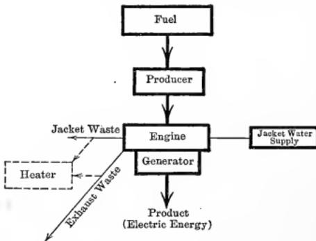
Fig. 443.—Elements of a Producer Gas Power Plant.
