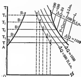
Fig. 44.— $T\phi$ -Diagram Showing P-Curves, and Q-Curves.
