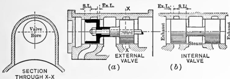
Fig. 150. — External and Internal Piston Valves.
