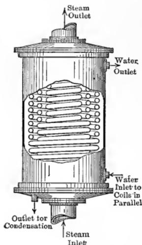
Fig. 423. Coil Heater.
