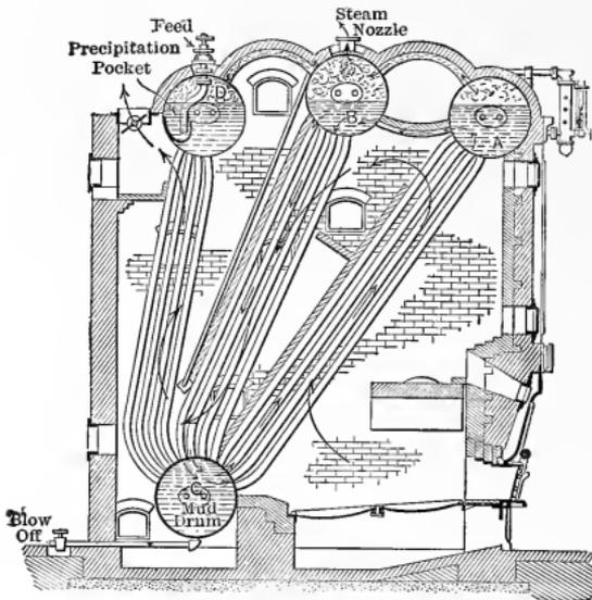
Fig. 363. — Stirling Type of Boiler.
