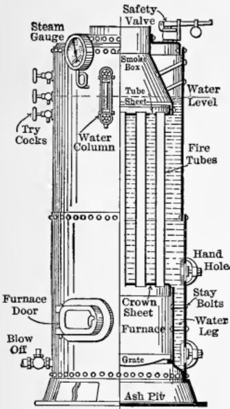
Fig. 352. — Tubular Boiler.
