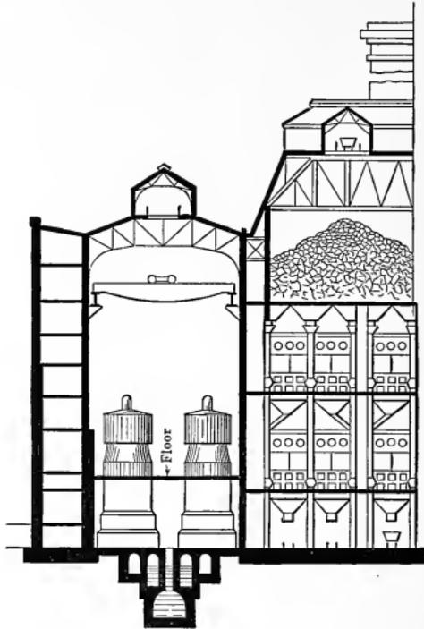
Fig. 448. — Power Plant with Double Deck Boiler Room.
