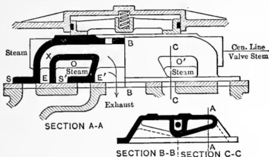
Fig. 151. — Double-ported Marine Valves.
