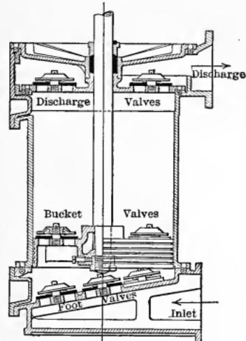
Fig. 438. — Wet Air Pump.
