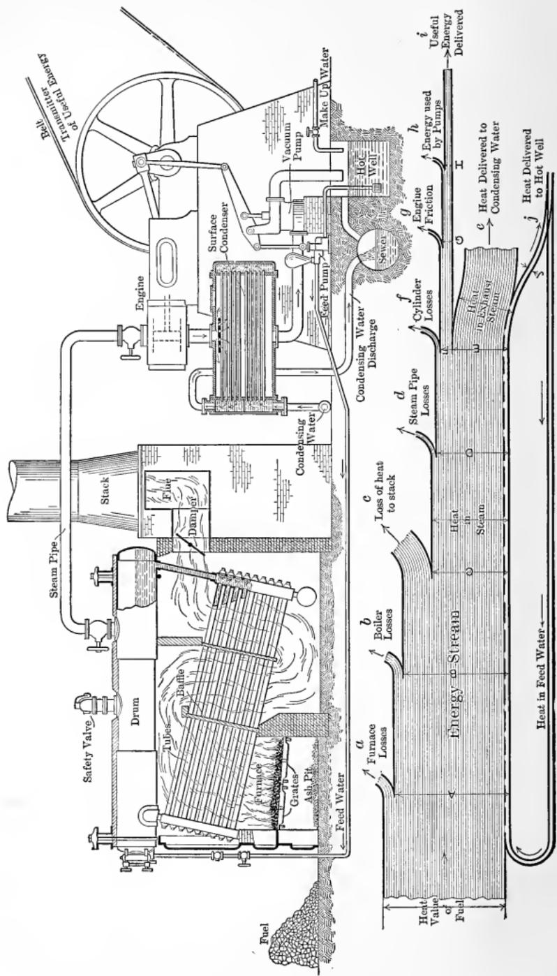
Fig. 3. — Elements of a Steam-Power Plant.
