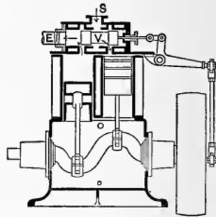
Fig. 102. — Vertical Twin-Cylinder, Single-Acting Engine.
