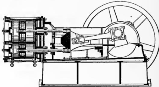
Fig. 109. — Duplex-Compound Engine.
