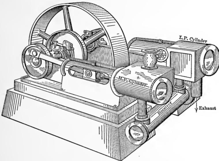
Fig. 108. — Cross-Compound Engine.
