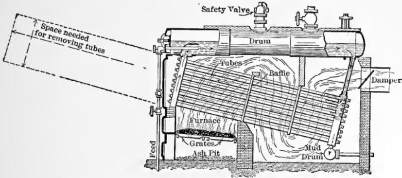
Fig. 361. — B. and W. Type of Boiler.
