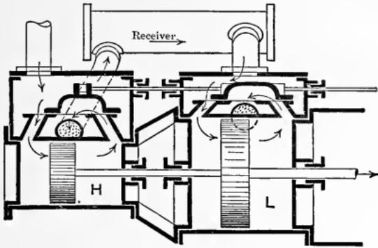
Fig. 107. — Tandem-Compound Cylinders.
