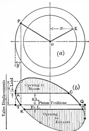
Fig. 139. — Elliptical Diagram.
