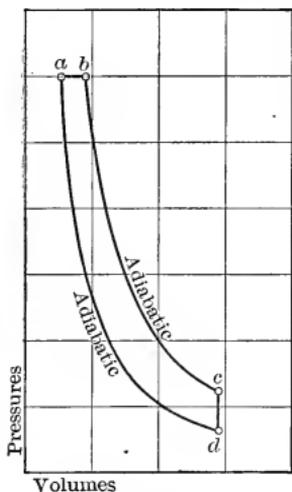
Fig. 29. — PV-Diagram of Diesel Cycle. Air as working substance. The lines bc and cd coincide with the lines similarly lettered in Fig. 26.
