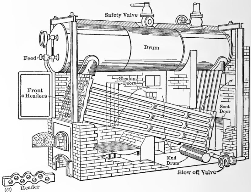
Fig. 360. — B. and W. Type of Boiler.
