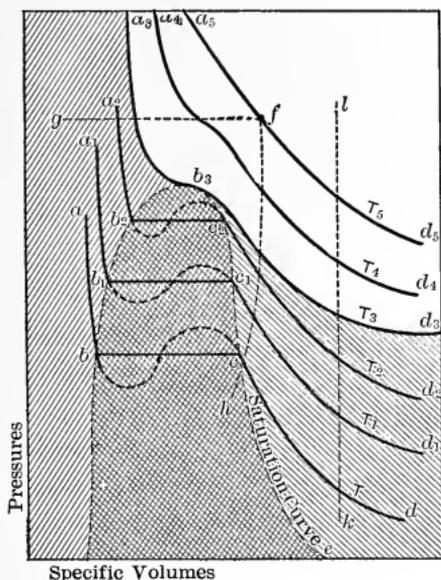
Fig. 34.—Isotherms of Material in Liquid, Vaporous and Gaseous States.
