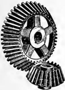
Fig. 208. Bevel gearing.
