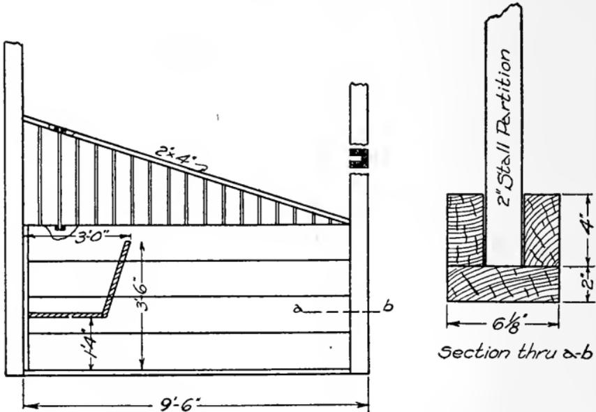
Fig. 286. Detail of construction of a horse stall.
