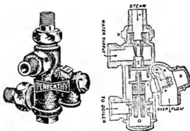
Fig. 245. A standard type of injector.
