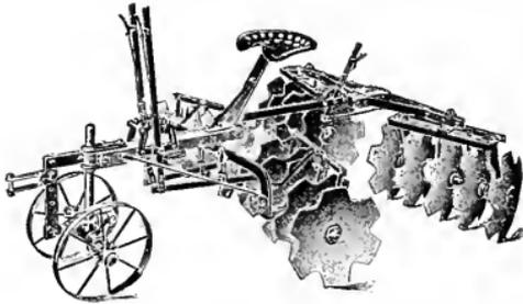
Fig. 124. A cutaway disk harrow.
