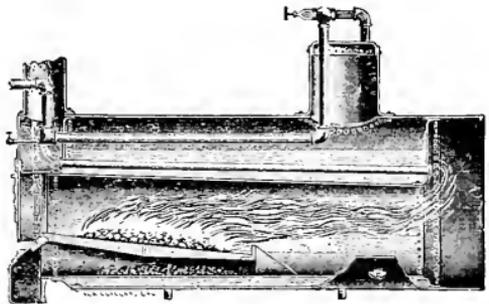
Fig. 242. A sectional view of a return-flue boiler.
