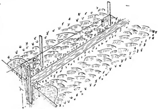
Fig. 56. The line method of grading tile ditches.
