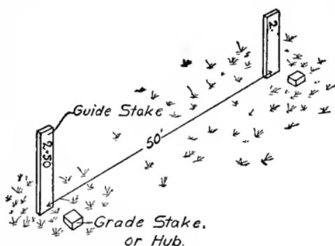
Fig. 49. Grade stakes, or hubs, and guide stakes.
