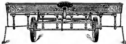
Fig. 136. A broadcast seeder with a narrow-track truck.
