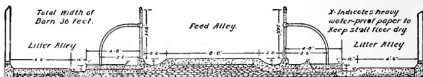
Fig. 283. Cross section through stalls in a modern dairy barn.
