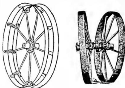
Fig. 146. The open and double type of corn planter wheels.
