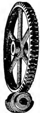
Fig. 209. Worm gearing.
