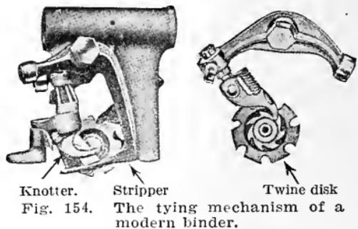
the failure to make a complete knot. The names of the various parts of the tying mechanism may be learned from the accompanying illustration. If the needle does not carry the twine over far enough, the twine disk, or cord holder, will grasp only one strand, and the knot will be tied only
