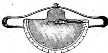
Fig. 198. A direct-reading traction dynamometer.
