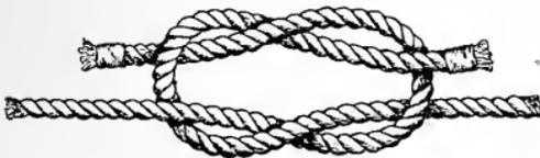
Fig. 326. Granny knot, or false reef.
