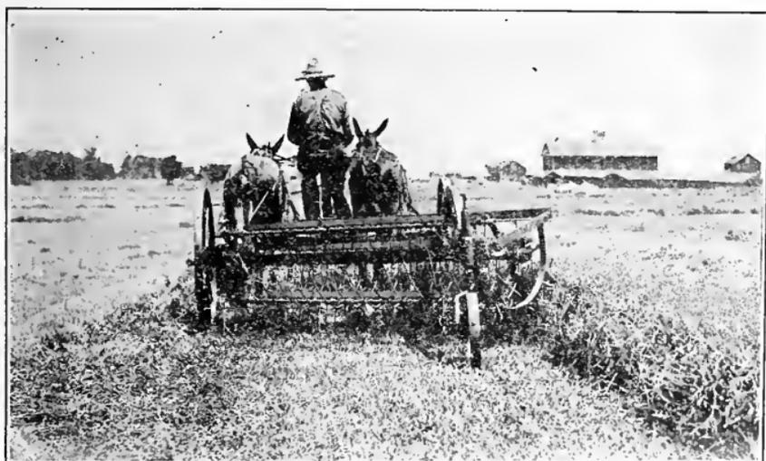
Fig. 166. A three-bar side-delivery rake at work.
