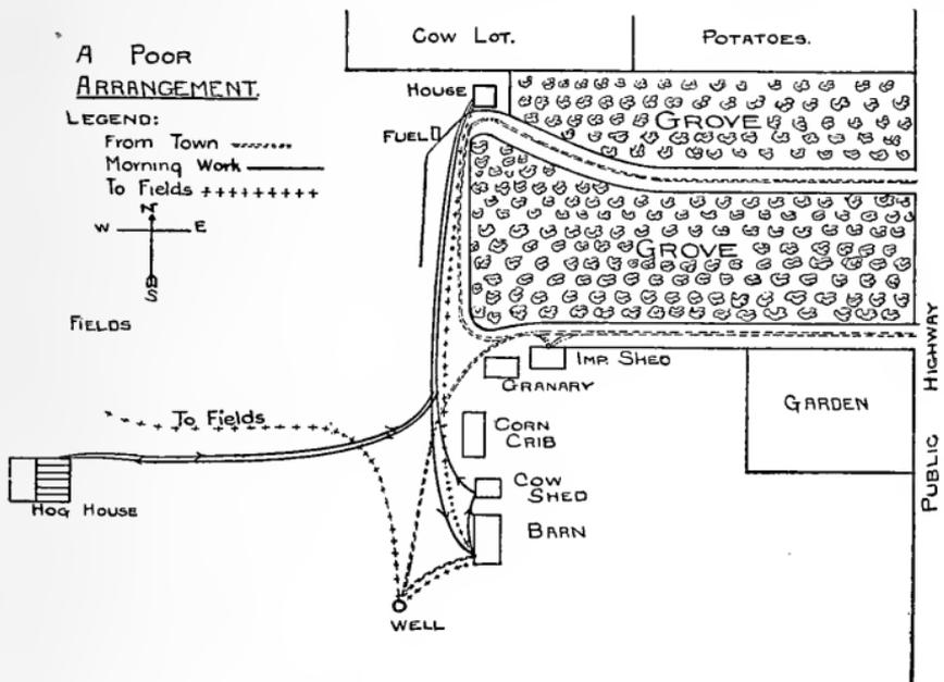
Fig. 253. An inconvenient arrangement of farm buildings.
