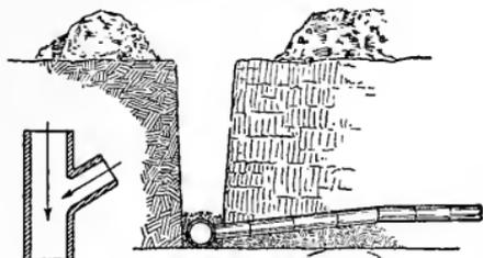
Fig. 60. Sketches showing proper method of joining lateral drains to mains. From Ohio Exten. Bul. 47.
