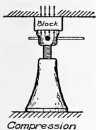
Fig. 256. A sketch illustrating a compressive stress.
