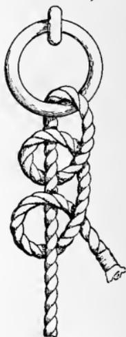
Fig. 335. Two half hitches.
