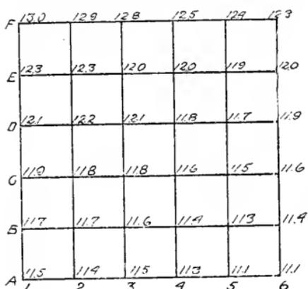
Fig. 39. Plat showing how levels may be taken over an entire field. The stations are indicated by letter and numbers, as B<sub>2</sub>, etc.
