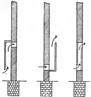
Fig. 323. Different methods of arranging the inlet flues in the King system of ventilation.
