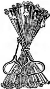
Fig. 1. The Gunter's chain, folded.
