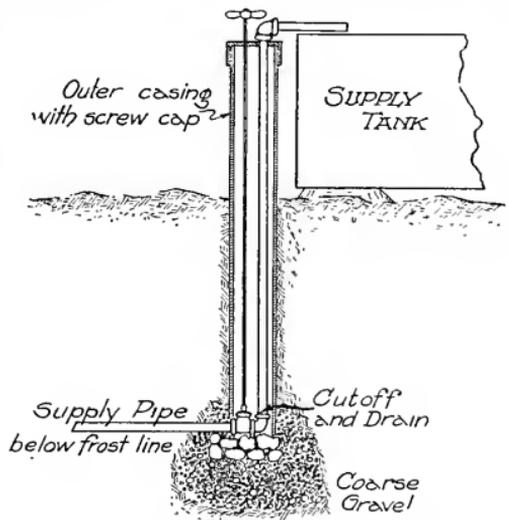
Fig. 306. A satisfactory method of installing exposed hydrants.
