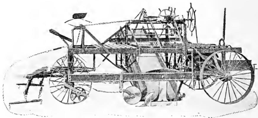
Fig. 92. An elevating grader.
