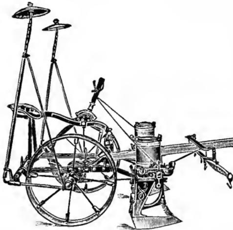
Fig. 144. A corn planter with stub shoe furrow-openers.
