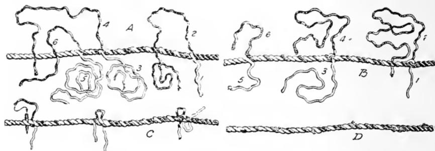
Fig. 340. Long splice, three-strand rope.
