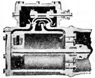
Fig. 247. A sectional view of the cylinder and steam chest of a simple engine.
