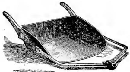
Fig. 87. Scoop scraper or slip.
