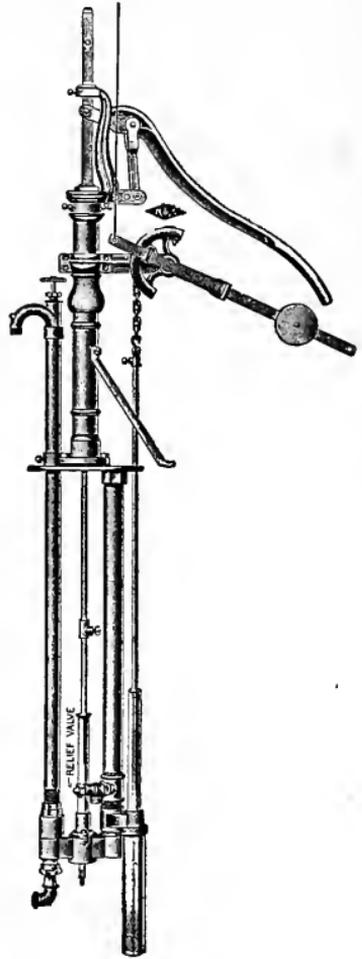
Fig. 302. A good type of three-way or underground pump. This pump is provided with a hydraulic cylinder to throw the windmill out of gear when a certain pressure has been reached.
