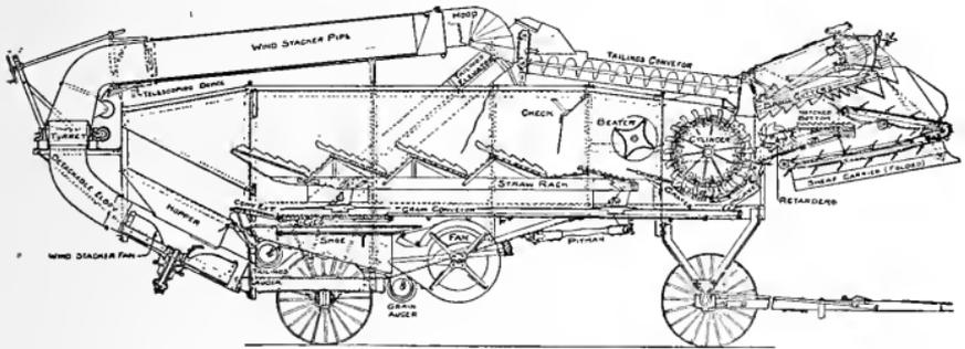
Fig. 177. A section of a modern threshing machine.
