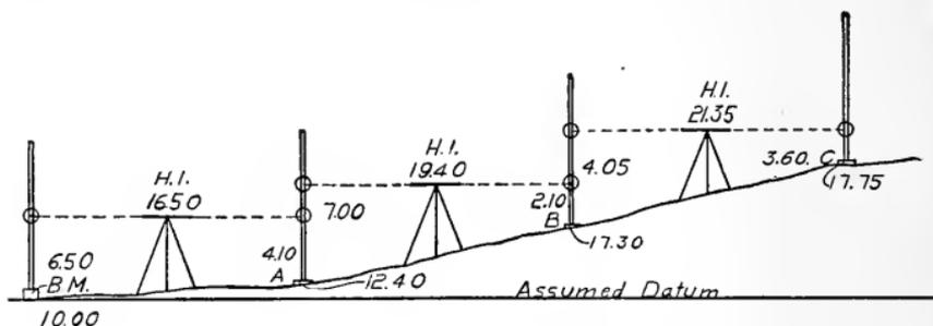
Fig. 38. Sketch illustrating the levels of Fig. 37.
