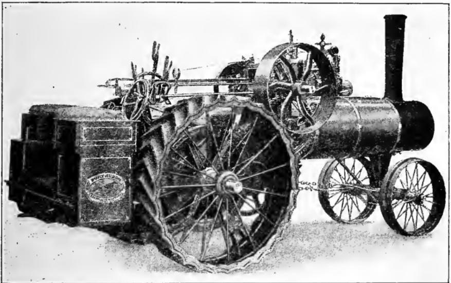
Fig. 252. A top-mounted steam tractor.
