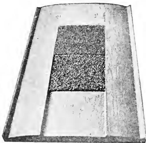
Fig. 85. Model of a water-bound macadam road. *A* represents the prepared subgrade. *B* represents the first course of coarse stone. *C* represents the second course of stone, and *D* the finishing layer of stone, chips or dust. (Bul. 36, Office of Public Roads, U. S. Dept. of Agr.)
