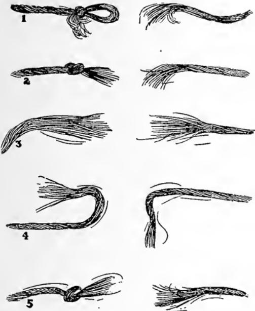
in one end of the cord, with the other extending back to the machine. This condition is shown in No. 1, Fig. 155, and may be caused occasionally by a straw interfering with the placing of the twine.
