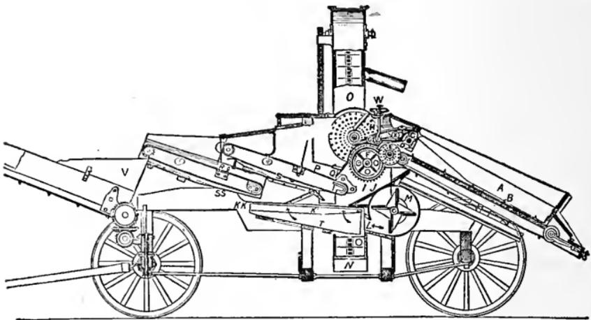
Fig. 190. A section of a picker-wheel sheller.
