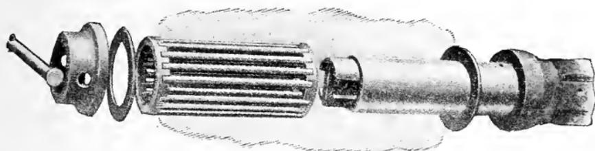
Fig. 103. A roller bearing for wagons. The hub of the wheel fits over the rollers shown.
