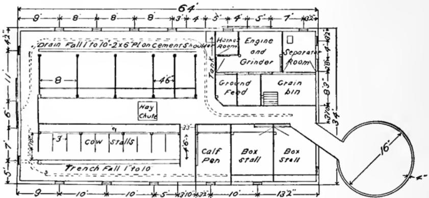
Fig. 284. Floor plan of a general farm barn.
