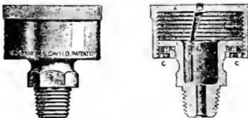
Fig. 107. A grease cup for feeding hard oil.
