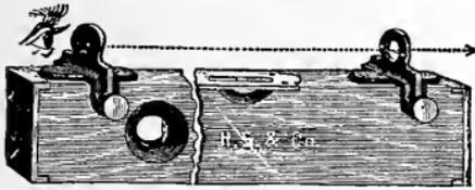
Fig. 33. A carpenter's level with sights attached.
