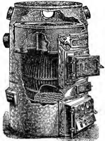
Fig. 319. A typical warm-air furnace.
