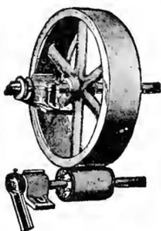
Fig. 210. Friction gearing.
