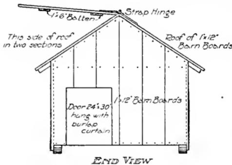
Fig. 265. End elevation of gable-roof colony hog house.
