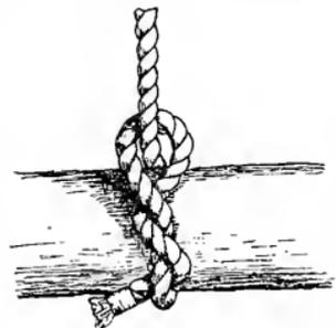
Fig. 333. Timber hitch.
