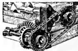
Fig. 211. A link belt or chain transmissions.
