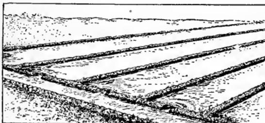
Fig. 75. Border method of irrigation.
