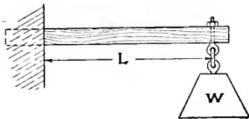
Fig. 258. A sketch showing a cantilever beam, or a beam fastened solidly at one end, and the action of a load at the free end.
